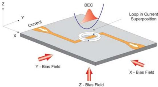
Fig. 1: Schematic of an atom chip containing the superconducting loop.
