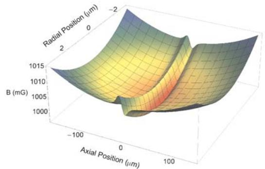
Fig. 2: Perturbation induced in the magnetic trap by the loop in state  $|0\rangle$ .
