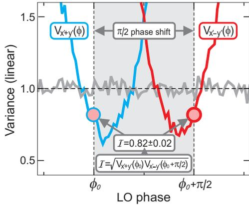
Fig. 1: Results for inseparability. Measurement of the variance for the sum  $V_{x'+y'}(\phi)$  and difference  $V_{x'-y'}(\phi)$  for the  $45^\circ$  rotated fields. The data, both below the QNL, are combined to one value for the inseparability of  $\mathcal{I} = 0.82 \pm 0.02$ , demonstrating significant entanglement between two orthogonal spatial modes within one optical beam.
