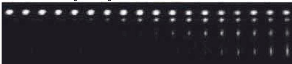
Figure 1. Experimental data showing Rabi cycling between the magnetic hyperfine states of the  $5^2S_{1/2} F = 2$  manifold of  $^{87}\text{Rb}$ . For each individual data set a  $50 \mu\text{s}$  pulse of Raman coupling is applied to a trapped BEC, followed by a free evolution time of 5 ms and absorption imaging. The images show the BEC atoms coherently Rabi cycling between the separately resolved magnetic sub-states as we increase the laser power in the Raman pulse.
