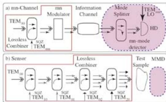
Figure 1: Schematic layout for a multi channel optical system. a) shows the components we have built and tested for a communication network. b) shows a spatial sensor.
