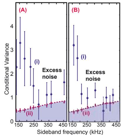
Conditional variance in the (A) amplitude and (B) phase quadratures. The data point groups show (i) EIT and (ii) passive loss conditional variance. The passive loss benchmark was simulated by using a variable beamsplitter to match the EIT transmission
