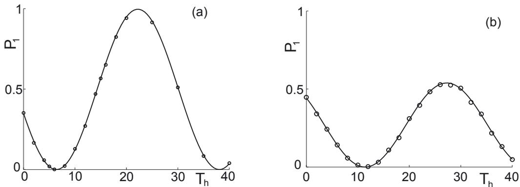
Figure 1. Dependence of the first excited state population  $P_1$  on the duration of the holding stage  $T_h$  for various splitting and recombination stages with  $T_s = T_r = 20$  (a), 200 (b). Results of the Bloch vector model are represented by solid lines and those of the full numerical simulations are presented by circles.  $T_s$ ,  $T_r$  and  $T_h$  are in units of the vibrational frequency of the original potential well.
