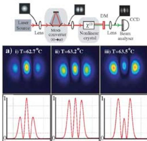
Figure 1: mode conversion for the case of simple pass SHG in a Lithium Niobate for three different crystal temperatures
