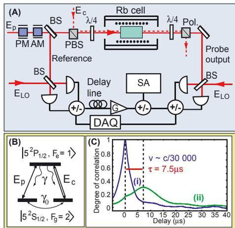
(A) Experimental schematic. (B) Atomic level scheme used in the experiment. (C) Correlation plots showing a  $7.5 \mu\text{s}$  delay of a noise modulation (bandwidth 60 kHz) between the input (i) and output (ii).
