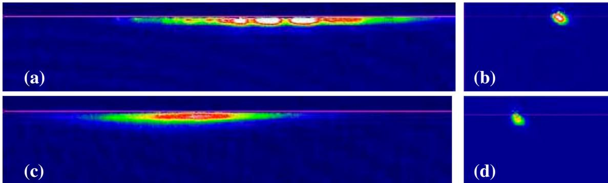
Figure 1. Absorption images of the atomic cloud positioned  $50 \mu\text{m}$  below the TbGdFeCo film in the axial (a) and radial (b) directions and  $50 \mu\text{m}$  below the gold film in the axial (c) and radial (d) directions. Fragmentation of the cloud in the axial direction is clearly visible below the magnetic film.
