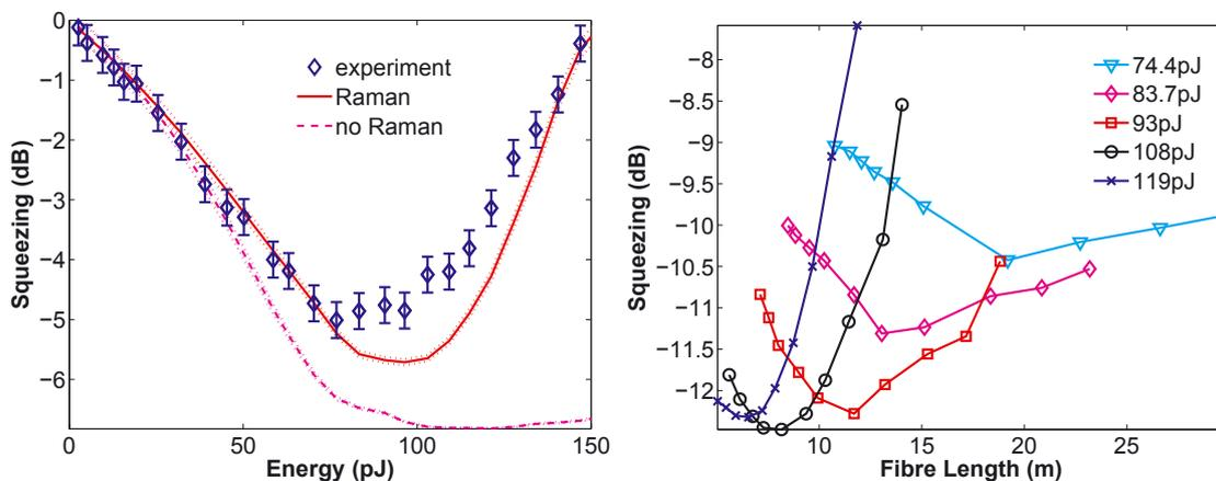
**Left:** Comparison of simulations and experiment for  $L = 13.35\text{m}$ . Dashed line is the simulation with a fully electronic nonlinearity (i.e. no Raman effects). **Right:** Predicted optimum squeezing for various fibre lengths. Parameters:  $t_0 = 74\text{fs}$ ,  $z_0 = 0.52\text{m}$ ,  $\bar{n} = 2 \times 10^8$ ,  $E_s = 54\text{pJ}$ ,  $\lambda_0 = 1.51\mu\text{m}$ , linear losses 20%.
