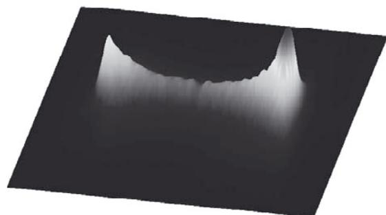
Figure 1: Image of an atom laser beam outcoupled from the centre of the BEC. Note the appearance of caustics at the edge of the beam. The size of the image is  $1 \text{ cm} \times 1.3 \text{ cm}$ .
