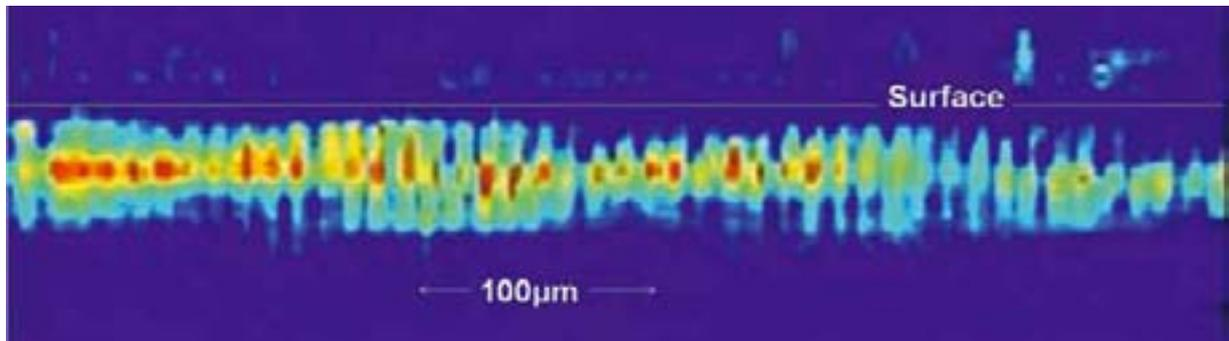
Fig. 1: Fig. 1: Sideview *in situ* absorption image of  $^{87}\text{Rb}$   $F=1$  atoms trapped in a  $10\ \mu\text{m}$ -period 1D magnetic lattice. (Pixel size:  $3\ \mu\text{m}$ .)
