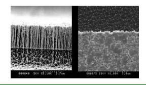
Orsay 2<sup>nd</sup> generation: 700 nm width evaporated gold wires, pattern written with e beam
