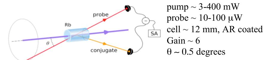
probe and conjugate polarization orthogonal to pump
