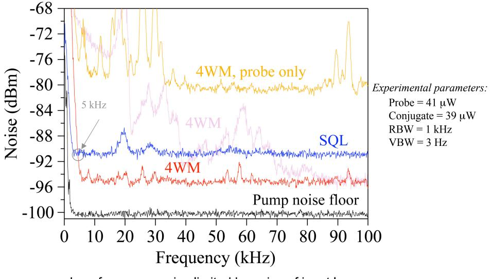
Low-frequency noise limited by noise of input laser.
