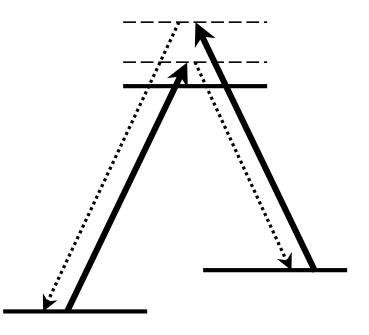
4WM based on ground-excited coherences and ensuing absorption and spontaneous emission noise Slusher, et al., 1985
